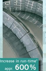
Our Rotors and screw presses are manufactured exclusively from highalloy special steels. The individual rotor blades just as the helix of screw presses are equipped with replaceable tool carriers with anti-wear layer which can easily be exchanged providing the possibility of a quick and simple replacement on demand.
